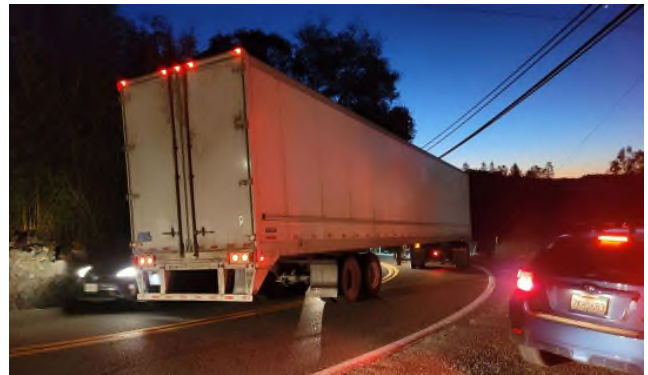
FIGURE 53: OVERSIZE TRUCK TRACKING INTO OPPOSITE LANE
