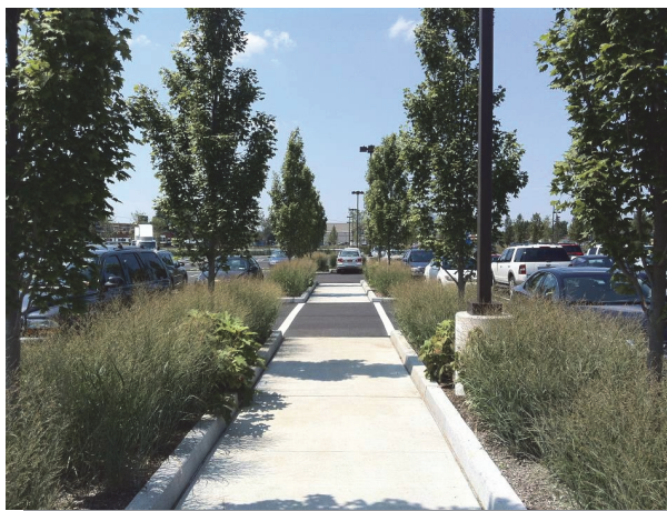
Shaded and planted walkways through parking lots provide safe, enjoyable routes to store entrances. They can also incorporate storm water treatment swales.
