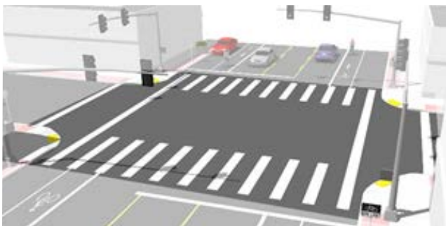
Figure 6-7: Example of high-visibility crosswalk markings
