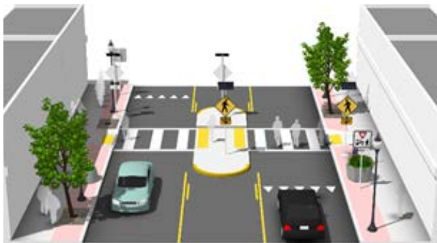
Figure 6-9: Example of an RRFB
