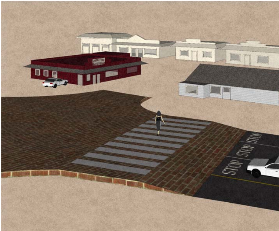
Figure 8. Raised intersection in Cool (rendering by Victor Tran)
