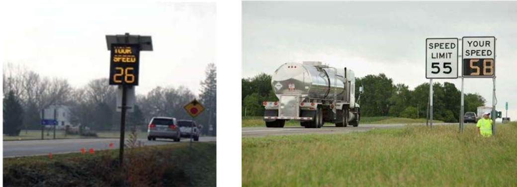
Figure 6. Speed feedback signs (FHWA)
